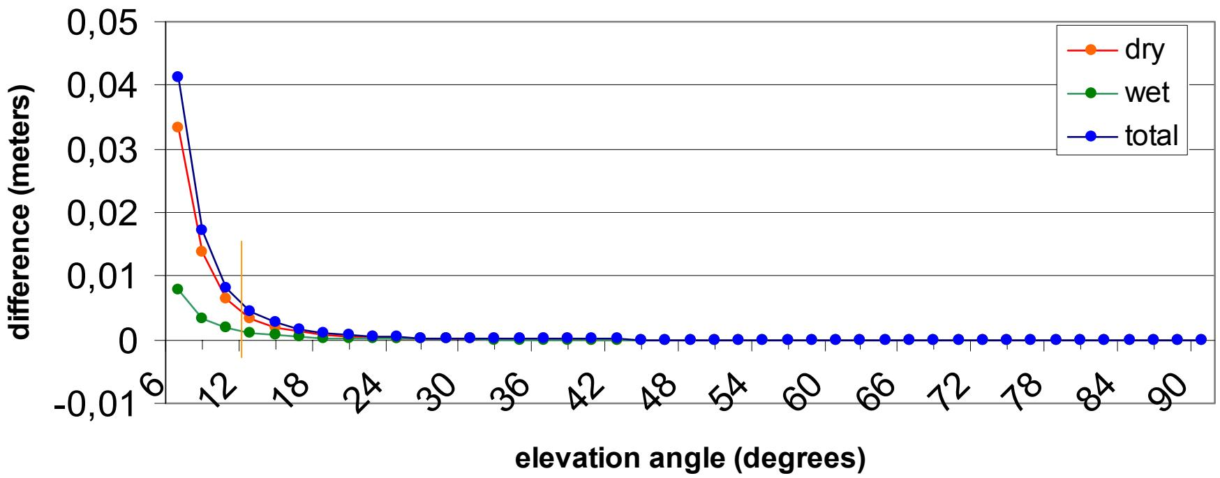
$$\text{ZTD} \quad \Delta L^z_d = 2.239 \text{ m} \quad \Delta L^z_w = 0.267 \text{ m}$$
