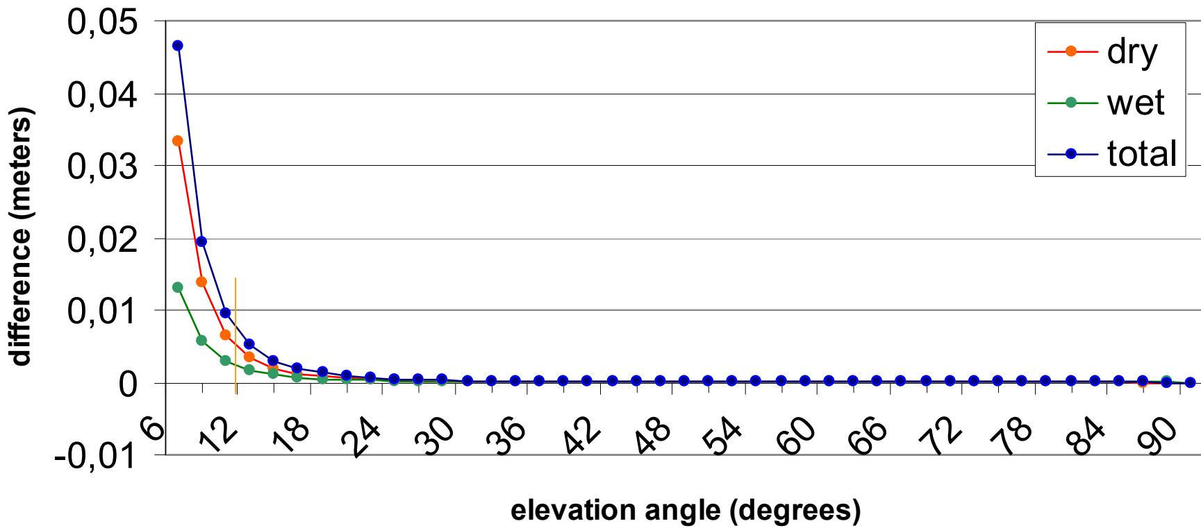
$$\text{ZTD} \quad \Delta L^z_d = 2.239 \text{ m} \quad \Delta L^z_w = 0.448 \text{ m}$$
